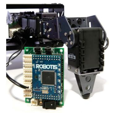
I am using the Robotis CM-700 controller to drive my AX12-18 Smart Hexapod. The controller is very robust and works well for standalone applications.
